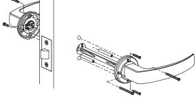
To attach furniture to the door fit the threaded spindles to one side of the backplate first then insert the square spindle with the scalloped side facing the grub screw in the handle. Then fit the other handle. Screw the machine screws into the threaded spindles. Tighten the grub screws in the handles. Then add extra wood screws for strength.
