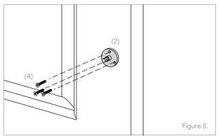
**3.4.** Place pull handle on taylor spindles and tighten both grub screws to secure.
