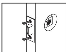
Insert Latch and Tighten Screws
