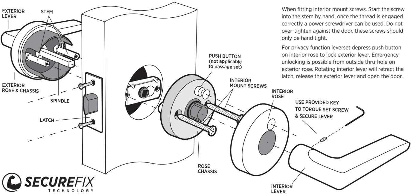
When fitting interior mount screws. Start the screw into the stem by hand, once the thread is engaged correctly a power screwdriver can be used. Do not over-tighten against the door, these screws should only be hand tight.
