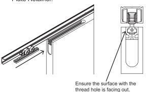
(b) To adjust the panel height, firstly remove the hanger plate out from the retainer on panel and then rotate the hanger bolt by using the Allen key: clocksize to lower; anticlockwise to raise.
