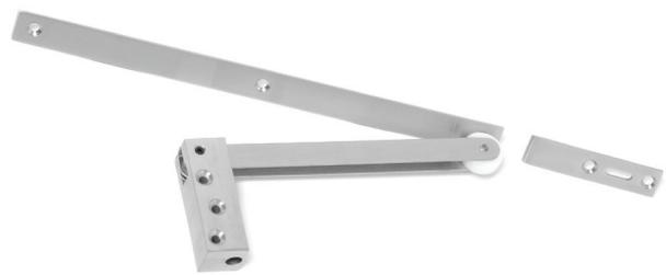
Briton Door Coordinators are designed for use on pairs of doors, where the inactive is required to close before the active leaf. The door selector is suitable for double rebated doors and fire doors. Door coordination is a basic requirement for all self-closing pairs of doors that are rebated or have astragals.
