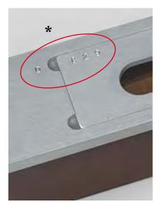
The routing templates (A &B), which comprise of a frame and two inserts, enables the drilling/ routing of two slots for the invisible hinges body, the templates are made from 5 mm thick aluminium plates.
