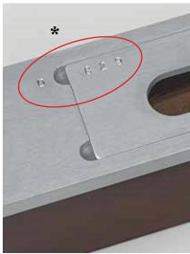
The routing templates (A &B), which comprise of a frame and two inserts, enables the drilling/ routing of two slots for the invisible hinges body, the templates are made from 5 mm thick aluminium plates.
