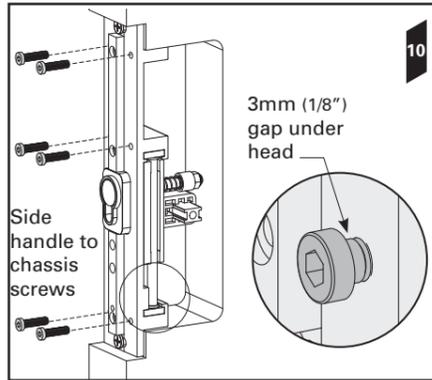
**11.** Fit the *privacy side handle* containing the snib latch to the chassis as follows (if installing a snib/snib privacy handle install **ONE** of the side handles only):
