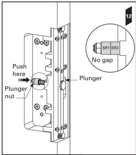
**13.** Two identical spanners have been supplied. Restrain the *plunger nut* using the **large** end of one of the supplied *spanners*. Place the **small** end of the second spanner across the flats under the head of the plunger. Keep the spanner restraining the plunger nut **stationary** while turning the second spanner **clockwise**.
