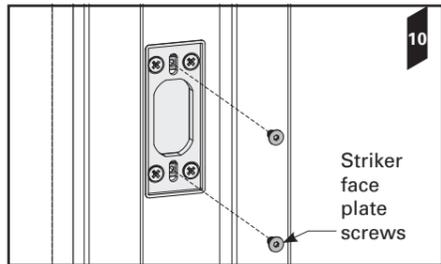
**11.** Position the *striker face plate* in the centre of the *striker body* - this may need to be adjusted in the steps following. Insert the *striker face plate screws* and loosely tighten.
