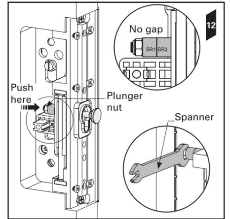
**13.** Two identical spanners have been supplied. Restrain the *plunger nut* using the **large** end of one of the supplied *spanners*. Place the **small** end of the second spanner across the flats under the head of the plunger. Keep the spanner restraining the plunger nut **stationary** while turning the second spanner **clockwise**.
