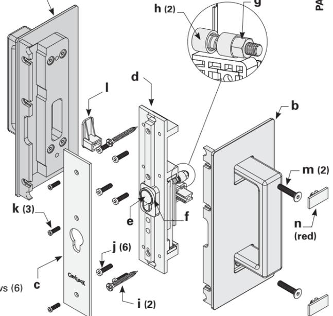
**Note: Components will vary between the 'Snib/Emerg', 'Snib/Snib' and 'Snib One Side' versions. Straight handle option shown.**
