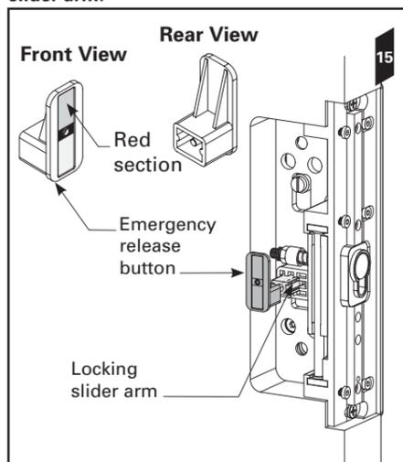
**Fitting the Remaining Side Handle and Face Plate**
