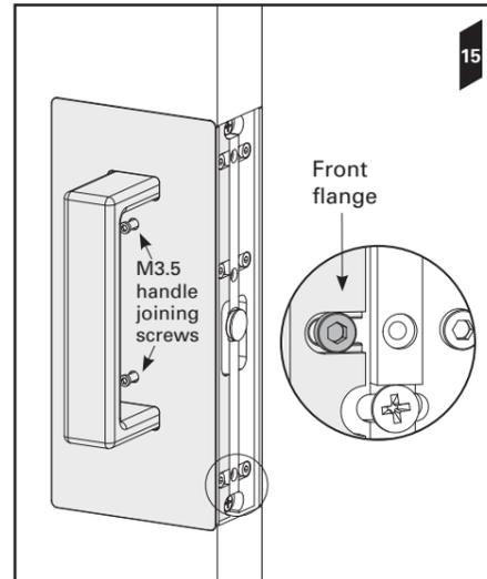
**16.** Use the ball end of the *CL400 Allen key* to fasten the 2x *M3.5 screws* as tight as possible. Use the other end of the Allen key to fully tighten the screws. **It is important that they are tight.**
