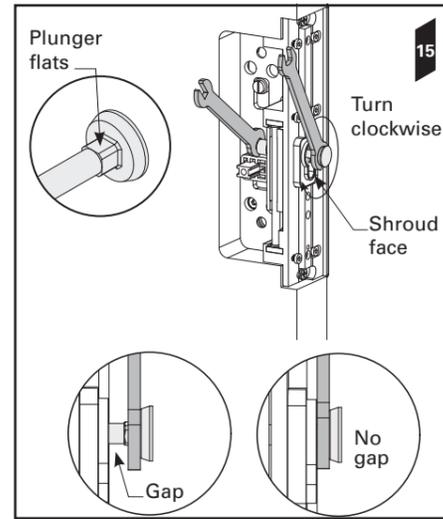
Now turn the *spanner* **anti clockwise** half a turn. The *plunger* should now be adjusted correctly. Slide the door closed to check that it latches. If the *snib* button is hard to push down or the *plunger* doesn't engage with the *striker*, adjust as necessary.
