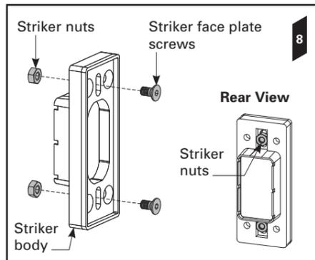
**9.** Insert the *striker body*, with the *striker face plate screws* and the *striker nuts* attached, into the cut out in the closing jamb.
