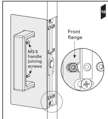
**17.** Use the ball end of the *CL400 Allen key* to tighten the 2x handle joining screws.
