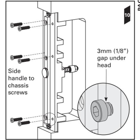
**11.** Fit the *passage side handle* (with no visible fasteners) to the chassis by sliding the front flange of the handle under the heads of the 3x *side handle to chassis screws*. Tighten the screws.
