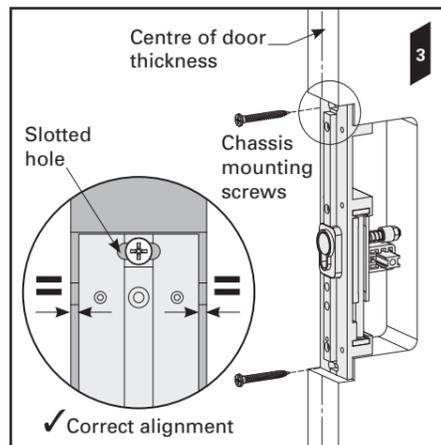
4. Fit the 6x *side handle to chassis screws*. Leave a 3mm (1/8") gap between the underside of the screw head and the chassis.
