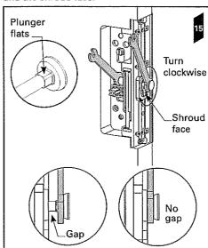
Now turn the spanner anti clockwise half a turn. The plunger should now be adjusted correctly. Slide the door closed to check that it latches. If the snib button is hard to push down or the plunger doesn't engage with the striker, adjust as necessary.
