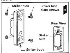
9. Insert the striker body, with the striker face plate screws and the striker nuts attached, into the cut out in the closing lamb.
