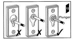
13. The striker allows 2.5mm (3/32") of adjustment in each direction when the striker face plate is fitted in the centre of the striker
