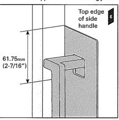
Open the door. Transfer the horizontal line across the centre of the closing jamb. This line represents the top of the striker cut out. A double-sided striker cut out template has been provided:
