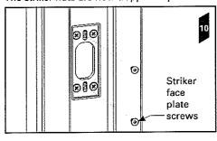
11. Position the striker face plate in the centre of the striker body - this may need to be adjusted in the steps following. Insert the striker face plate screws and loosely tighten.
