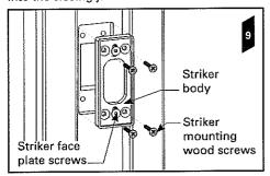
Remove the striker face plate screws. The striker nuts are now trapped in position.
