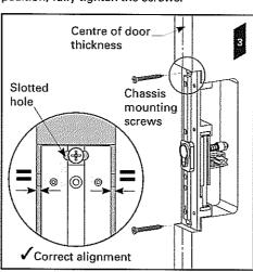
Fit the 6x side handle to chassis screws. Leave a 3mm gap (1/8") between the underside of the screw head and the chassis.
