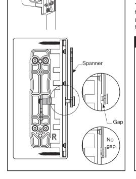
**17.** Use the ball end of the *CL400 Allen key* to tighten the 2x handle joining screws. Use the other end of the Allen key to firmly tighten the screws.
