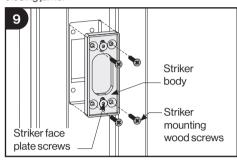
**10.** Remove the striker face plate screws. The striker nuts are now trapped in position.
