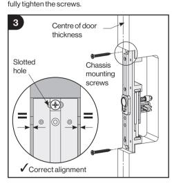
Fit the 6x side handle to chassis screws. Leave a 3mm gap (1/8") between the underside of the screw head and the chassis.
