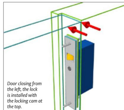
*Door closing from the left, the lock is installed with the locking cam at the top.*
