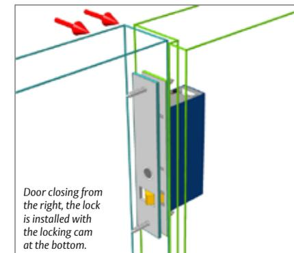
*Door closing from the right, the lock is installed with the locking cam at the bottom.*
