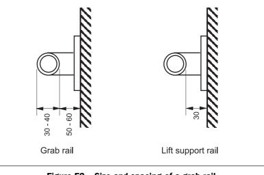
Figure F2 – Size and spacing of a grab rail
