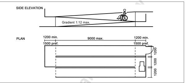
Figure 11 - Zigzag ramps: layout
