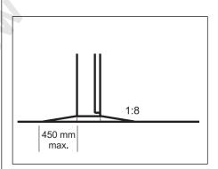
Figure 17 – Threshold ramp
