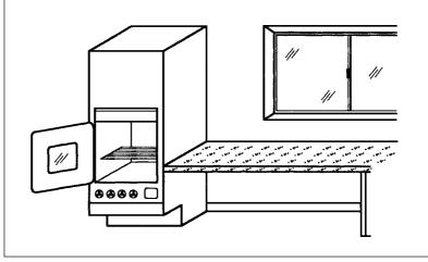
Figure 52 – Oven with worktop to allow for set-down
