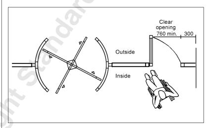
Figure 18 - Revolving door with side hung door
