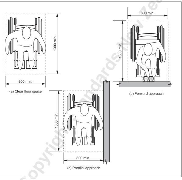
Figure D9 – Minimum clear floor space
