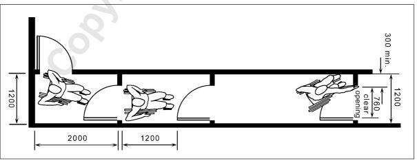
Figure 19 – Space requirements in confined spaces
