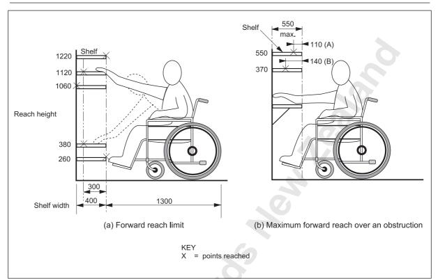
Figure D14 – Forward reach from a wheelchair
