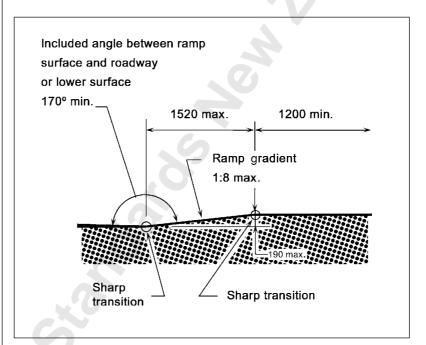
Figure 16 – Section through a step ramp
