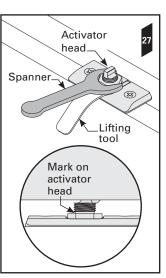
30. For units requiring Soft Open and Soft Close, repeat steps above to install a SofStop cassette at the other end of the track. Only one activator is required on the door.
