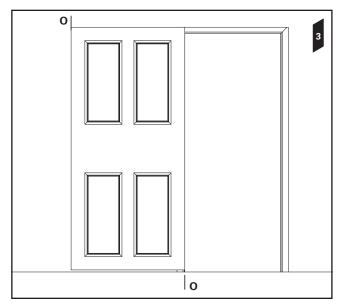
**4.** Manually position the door in the desired 'closed' position.
