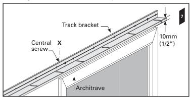
Level track bracket(s) by pivoting around central screw(s). Lock in place with two outer screws. The ends of double brackets should be touching. We recommend you clamp them together to keep them aligned for the next step.
