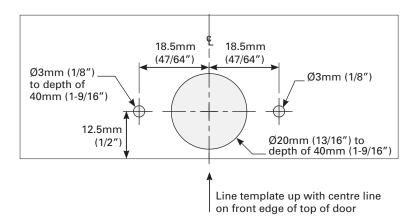
**Doors 810mm (32") or wider:** Mark a centre line on the top edge of the door, then mark and drill holes as shown below.
