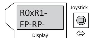
5. In the rest position, press in the joystick: Reset OK? ⇒ The relay PCB is deleted from the configuration.
