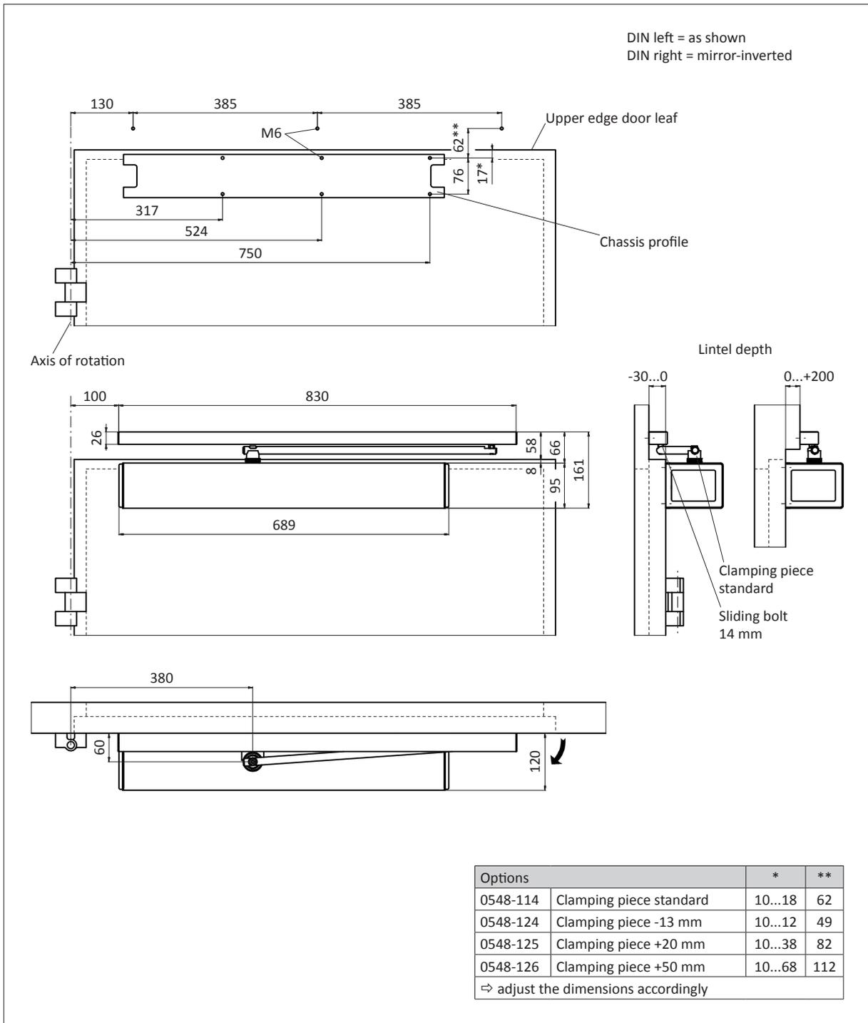
2. Mount the drive mechanism.
