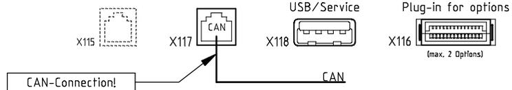
Only for version "Inversed" with optional fire-protection PCB
