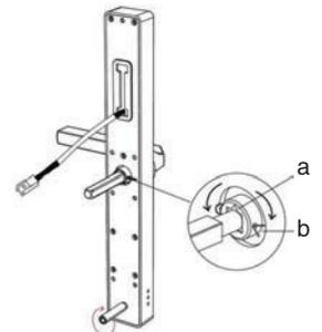
4. Fit the threaded sleeve to the bottom spigot by turning it counterclockwise and tighten it.
