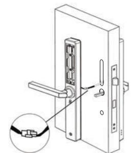
8. Hold the front panel against the door face, sliding the spindle and threaded sleeves through the drilled holes. Install the back panel by tightening the screws through the back panel into the threaded sleeves. Ensure the panels are sitting straight on the door.
