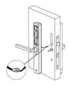
8. Hold the front panel against the door face, sliding the spindle and threaded sleeves through the drilled holes. Install the back panel by tightening the screws through the back panel into the threaded sleeves. Ensure the panels are sitting straight on the door.
