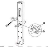
5. Insert the sliding threaded sleeve into the top shaft, choosing the correct height depending on the location of the mortice hole drilling. The sliding threaded sleeve can be adjusted between 55mm to 100mm to the centre of the square shaft.
