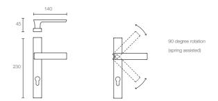
4 Point levers work with locks that throw bolts top and bottom, commonly used in aluminum joinery. This mechanism is available with all of our levers when using our long plate.
