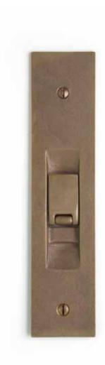
Mounted top or bottom, extension available with 20mm bolt offset, without extension bolt offsets available at 7.5,12.5,17.5 mm. Flip action provides an ergonomic grip. Offset options are measured from door edge to center of the bolt. Bolt is 5mm thick or 13mm round for the extension bolt. Weather proof strikes are available see Technical - Bolts page for options.
