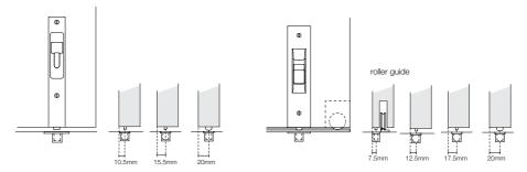
Offset options are measured from the door edge to the center of bolt
