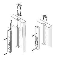
Installation top mount Slide Bolt with and with out extension
