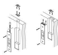
Installation top mount Flip Bolt with and without extension
