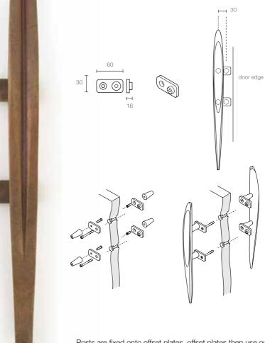
Posts are fixed onto offset plates, offset plates then use our standard through fixing
