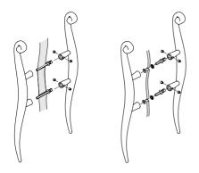
Pull handles as a standard come as a Back to Back Pair. We use a through fixing that is tightened up by grub screws on the internal handle.
