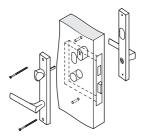
Lever on long plate with integrated turn, using an oval lock
