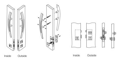
When installing note the top hole is for a half spindle, drill only half way through the door on the outside side, cut spindle down to suit door thickness
