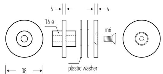
Halliday + Baillie brackets are tested in accordance with both the AS/NZS 1170.1:2002 (Structural Design Actions) standards and the International Building Code, IBC (2003) to comply with the 200lb fall rating.
