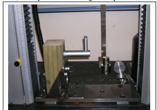
Fig 1 Jig used to apply compression loading to a HB 520 bracket assembly.
