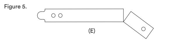
10. Place the inner rose privacy turn (B) over the spindle (D) from the inside of the door. \*For an accessibility turn, place privacy turn (B), with turn in the horizontal position, with flat spindle (E) through your privacy mechanism.
