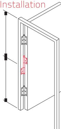
Install the spring hinge in the centre of the door between the two normal hinges.
