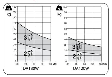
Based on a sliding scale, typical number of hinges per door starts at 2 increasing to 3 based on the graph above. For doors that require 3 hinges, please fit the 1st hinge at top, the 2nd placed 5cm below 1st hinge and the 3rd hinge at bottom.
