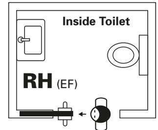
When standing looking into the cavity pocket, if the locking snib is on your **right hand** side then the LaviLock is a Right Hand lock.
