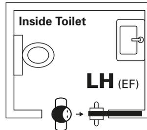
When standing looking into the cavity pocket, if the locking snib is on your **left hand** side then the LaviLock is a Left Hand lock.
