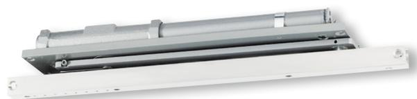
The LCN 6030 Series is a heavy duty non-handed, fixed strength, double acting, concealed overhead closer designed to fit in a narrow 44mm aluminium transom. The track arm and roller assembly, provides smooth, quiet door control. The closer cylinder is fitted in the aluminium frame, with the track fitted in the top rail of the door, providing complete concealment of the closer and it's arm.
