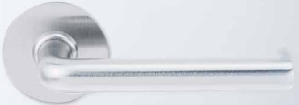
The 260 Series door furniture has a 55mm round rose. Concealed fixed plates have studs with internal threads located on the rose, visible roses have corresponding countersunk holes and are fixed back to back through the door.
