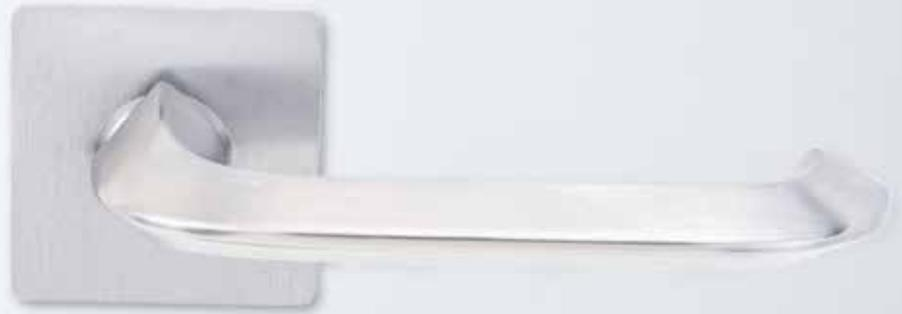
The 260SQ Series door furniture has a 55mm x 2mm square rose. Concealed fixed plates have studs with internal threads located on the rose, visible roses have corresponding countersunk holes and are fixed back to back through the door.
