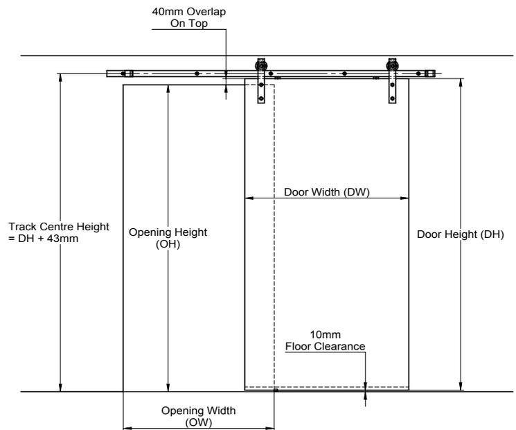
$$\text{Door Width (DW)} = \text{OW} + (2 \times 40\text{mm})$$
