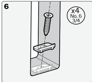
For wooden doors: install two woodfix brackets at top and bottom of cutout on the interior side of the door.
