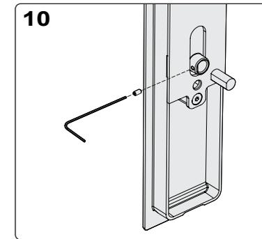
Select the correct spindle size from the guide on the contents page. Add a small amount of the supplied Loctite glue into the spindle hole. Insert spindle and secure with grub screw.
