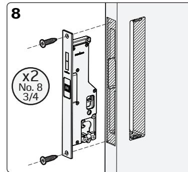
Insert the Euro Lock assembly and secure with two No. 8 3/4 screws.
