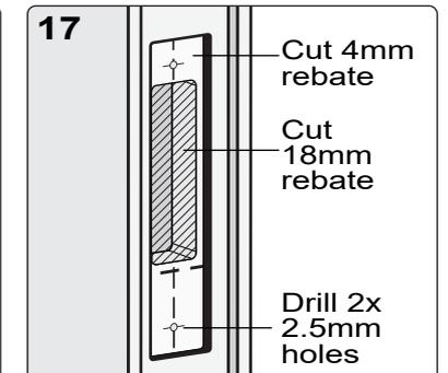
Place middle section of template into rebate and mark second rebate outline. Ensure it is the correct way up. Cut 18mm rebate. Mark screw holes and drill two 2.5mm holes 15mm deep.
