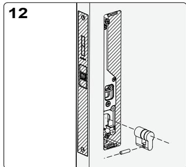
Insert locating pin (Grub Screw) into the Euro Lock cylinder and assemble into the Euro Lock body. Lock Cylinder supplied separately specific to door thickness. Note this is reversible for left/right opening doors.
