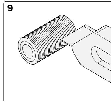
Trim the plastic spacer parts to fit the door thickness. Test fit and retrim if required.
