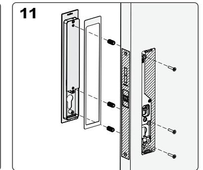
Insert the exterior lock flush pull handle with foam seal (For exterior use only) and trimmed spacer parts and secure with 3 x mounting screws. Refer to contents section for correct screw size.
