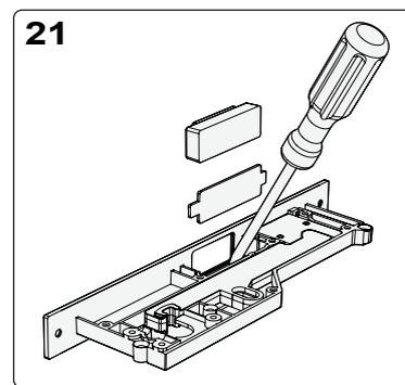
Using a flat screw driver remove the metal backing plate holding the rubber insert in place. Remove the rubber insert and slide the metal plate back in place. Reassemble the assembly plate and 6 screws.
