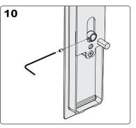
Select the correct spindle size from the guide on the contents page. Insert spindle into the flush pull with slide lock and secure with grub screw.
