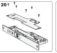
(Optional) Removal of the rubber insert to create a finger pull. Remove the 6 screws holding the assembly plate in place being careful not to remove any internal sliding components.
