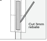
Remove middle section of end pull template and mark rebate outline on end of door. Use midline as height reference. Cut 3mm rebate.
