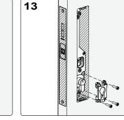
Secure the Euro Lock Cylinder in place with mounting bracket and 3 screws.
