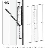
Remove middle section of striker plate template and mark outline for rebate. Use midline as height reference and ensure it lines up with the door. Cut a 4mm rebate.
