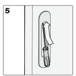
Use Mardeco hex tool to tighten grub screw inside top of flush pulls. Ensure they are fitted firmly.
