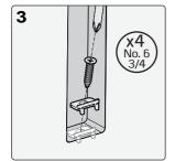
For wooden doors: install woodfix brackets at top and bottom of cutout.
