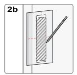
Aluminium Cutout: Match midline with template midline and position for desired backset. Mark aluminium cutout outline. Cut through aluminium.
