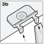
Fix bracket in centre of the cutout, ensuring that the tabs are hanging off the lip of the cutout. Once screw is fitted, snap off positioning tabs.
