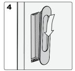
Insert flush pull into cavity. Push in and down so it grips onto the bottom bracket or edge.
