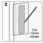
Wood Cutout: Remove middle section of flush pull template, position for desired backset and mark cutout outline. Use midline as height reference. Cut 13mm rebate
