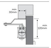
Top Jamb Installation Closer is fixed to the Top Jamb on the push (opposite to hinge) side of the door.
