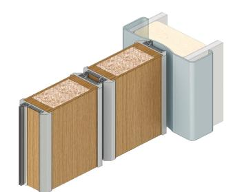
**Location:** Morticed into the door frame and around stiles and head.
