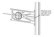
Remove factory fitted screws and studs from inside face of door rose. Discard these
