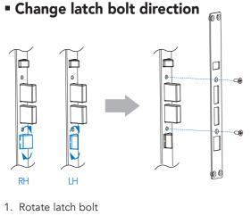
2. Confirm the direction of latch bolt and fix the plate using FH M4X10
