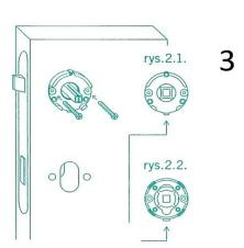
4 You can also stabilise the mounting adapters with wood screws.
