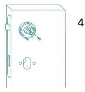
5 Push the spindle into the door lock or latch, with the notch facing downwards so that the spindle length is the same on both sides of the door.
