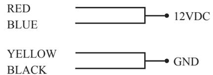
**4. Cabinet Lock Dual Voltage Wiring Diagram**
