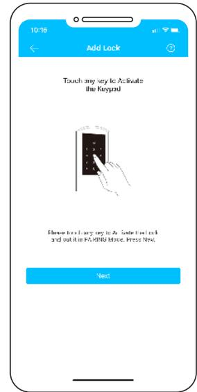
3. While standing near the lock (and with the 4 good quality AA alkaline batteries installed into the lock) wake the lock up by touching the key pad.
