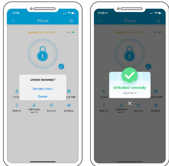
14. By clicking on the Wi Fi symbol, then clicking Remote unlock you will then be able to remotely unlock your lock from anywhere using the secure Wi Fi connection.
