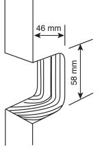
**1.** Decide on height of sliding pull handle on door. Using Template cut out detail in door.
