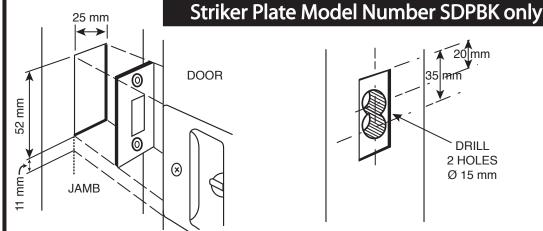
4. By closing the door, line up striker plate position on jamb, central to the lock. Mark and chisel out mortice for striker into the jamb.
