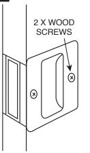
**3.** Fit sliding pull handle by tightening adjustment screws ensuring pull is central in the door. Fit the larger style wood screws as shown.
