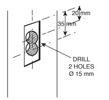
5. Drill two 15 mm (9/16") diameter holes, 12 mm deep at 20 mm from top of plate to centre of hole and also 35 mm from the top of the plate to the centre of the hole. Chisel out holes to form a rectangular hole for clearance of locking arm.
