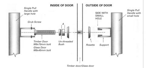
Working from the inside of the door, hold stainless steel rosette over the hole against the un-threaded bush onto the rosette, ensuring the larger section of the bush, as marked 'A' in above illustration, is facing the door.
