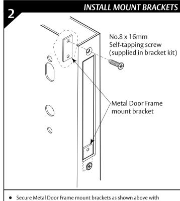
two of the No.8 x 16mm screws provided in the bracket kit.
