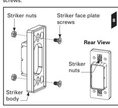
9. Insert the striker body, with the striker face plate screws and the striker nuts attached, into the cut out in the closing
