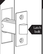
Insert latch with the curved side of the latch bolt facing in the direction that the door closes.
