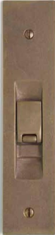
Mounted top or bottom, extension available with 20mm bolt offset, without extension bolt offsets available at 7.5,12.5,17.5 mm. Flip action provides an ergonomic grip. Offset options are measured from door edge to center of the bolt. Bolt is 5mm thick or 13mm round for the extension bolt. Weather proof strikes are available see Technical - Bolts page for options.
