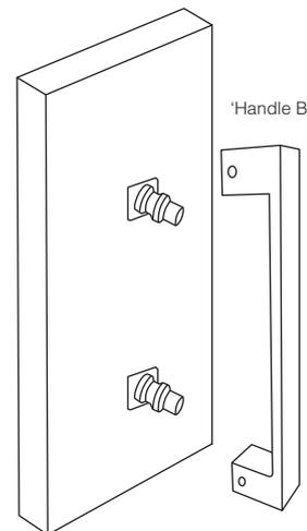
5. Insert 'Handle B' onto the brass mounts and secure it with the grubscrews.
