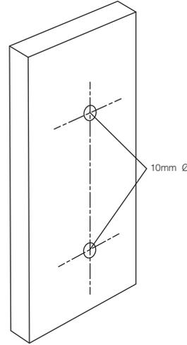
2. Mark the fixing position for the pull handle on the door. Ensure adequate space is provided for clearance of knuckles on the door jamb.
