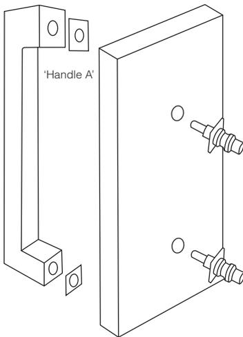
4. Screw the bolts through the door into 'Handle A' and tighten them.
