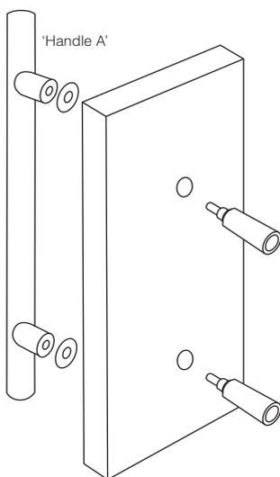
4. Insert the bolts through the legs and then through the door and tighten them onto 'Handle A'.
