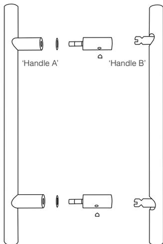
1. Take the pull handle apart by unscrewing the grub screws on both legs and then unscrewing the legs.
