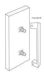
5. Insert 'Handle B' onto the brass mounts and secure it with the grubscrews.
