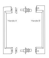
1. Take the pull handle apart by unscrewing the grubscrews on both legs and then unscrewing the bolts with a 5mm allen key.
