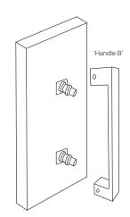
Insert 'Handle B' onto the brass mounts and secure it with the grubscrews.
