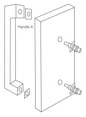
**4.** Screw the bolts through the door into 'Handle A' and tighten them.
