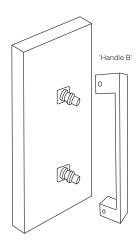
Insert 'Handle B' onto the brass mounts and secure it with the grubscrews.
