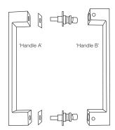
Take the pull handle apart by unscrewing the grubscrews on both legs and then unscrewing the bolts with a 5mm allen key.
