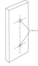
Mark the fixing position for the pull handle on the door. Ensure adequate space is provided for clearance of knuckles on the door jamb.
